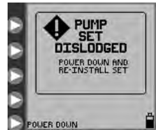
Figure 31. Pump Set Dislodged Error screen.
